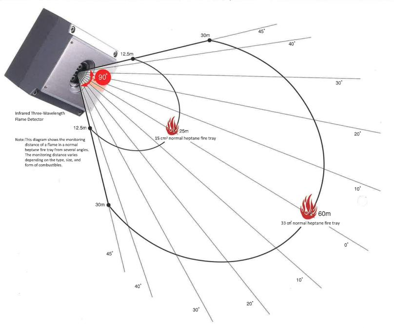
The PDCJ002-E detects the CO2 resonance radiation and flicker that are unique characteristics of flames. Despite its high sensitivity, the PDCJ002-E has fe er false alarm performance and can be installed under direct sunlight or artificial lighting such as sodium lamp, mercury lamp, fluorescent lamp, germicidal lamp, halogen lamp, etc.
