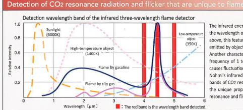
The infrared energy emitted from flames has the spectral characteristics of a peak in the wavelength of the 4.4µm band. This is called CO2 resonance radiation. As shown above, this feature is quite different from the spectral characteristics of infrared rays emitted by objects other than flames.
