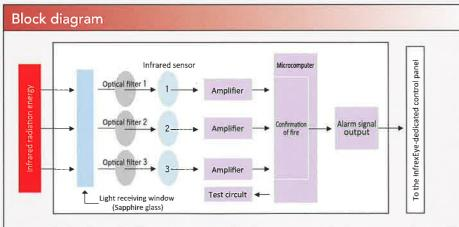
Nohmi's infrared three-wavelength flame detector (PDCJ002-E) is designed to detect the presence of fire from the radiant energy produced by flames (CO2 resonance radiation) and flame flicker. The PDCJ002-E quickly detects fire even in places with ventilation flow, external air, or high ceilings where detection is often difficult for the ordinary detectors. This high-sensitivity detector is suitable not only for large spaces but also for outdoor facilities.
