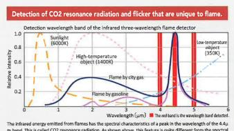
The infrared energy emitted from flames has the spectral characteristics of a peak in the wavelength of the 4.4µ m band. This is called CO2 resonance radiation. As shown above, this feature is quite different from the spectra characteristics of illndrared rays emitted by objects other than flames.
